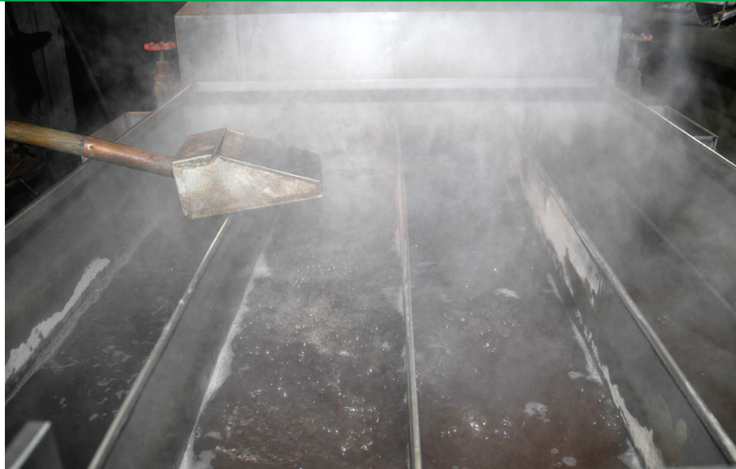
ABOVE: Sugar water flows into troughs where it is heated. The excess water evaporates, resulting in heavy syrup. It takes about 40 gallons of sugar water to produce one gallon of syrup.
