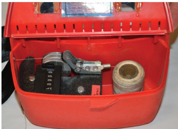
LEFT: As thread is pulled from the spool inside the stringbox, a wheel turns a counter to measure distance. The piece in the center, holding the wheel in place, is a simple drywall anchor. BELOW: The Chainman II stringbox kit includes directions and an extra spool of thread. The directions explain the reloading procedure.
