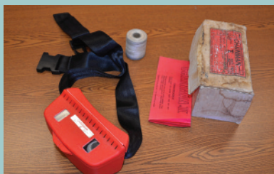
LEFT: As thread is pulled from the spool inside the stringbox, a wheel turns a counter to measure distance. The piece in the center, holding the wheel in place, is a simple drywall anchor. BELOW: The Chainman II stringbox kit includes directions and an extra spool of thread. The directions explain the reloading procedure.
