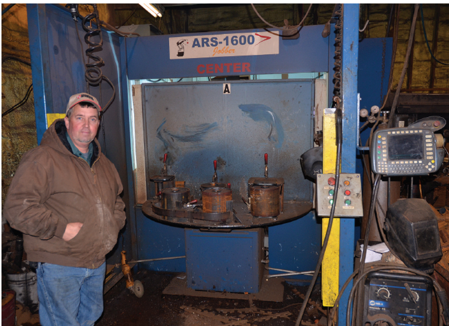
THIS IS HOW IT WORKS: Steve Stoltzfus explains how a computerized welder assembles rollers. Once the drums are positioned, on the near side of the machine, the table rotates to the back side of the machine for welding. Above, right: Once the bed of a container is assembled, it is moved by overhead crane through the rest of the assembly line. Right: The facility is nestled in the hills along Route 305.
