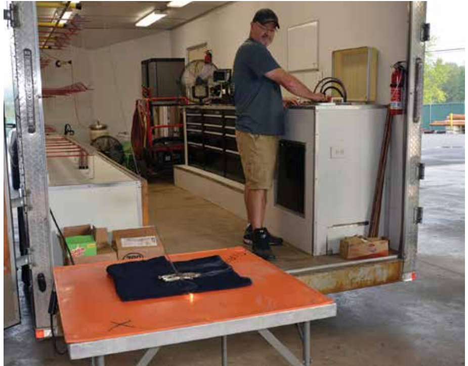
SAFETY CHECK: John Summers, owner and general manager of Versatile On-Site Laboratory Testing Services (VOLTS), LLC., tests a rubber blanket. To conduct the test, the orange blanket is spread out on an energized metal table and a wet and grounded towel is placed on top of it. The spark in the center of the table indicates a tear or puncture in the blanket.
