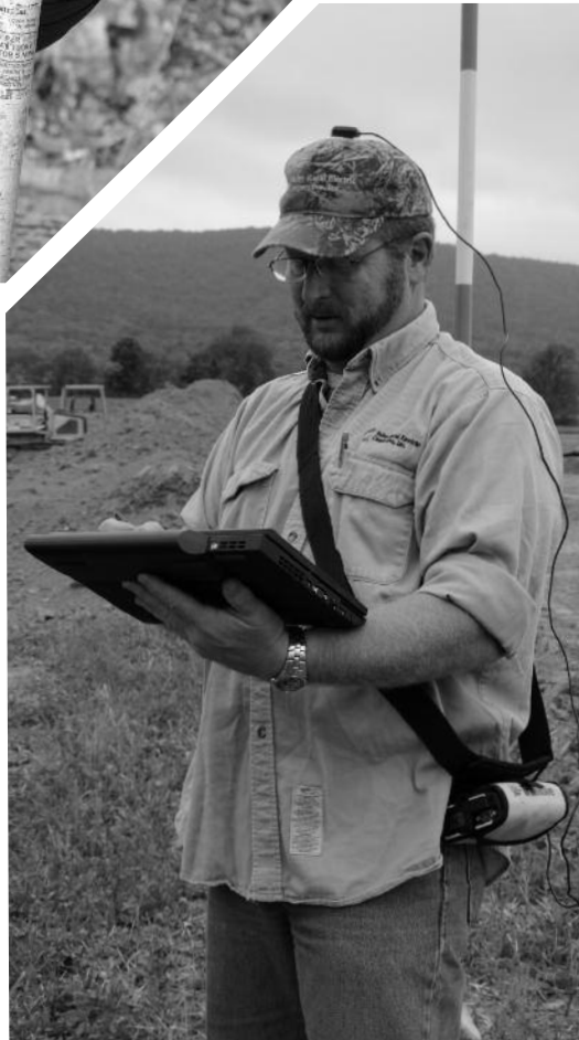
Above: Staking engineer Jason Hey uses a transit to select the route of a new line through a right-of-way. At right: Mike Lansberry uses GPS technology to plot a service drop to a turkey barn being built near Marklesburg, Huntingdon County in September. The GPS antennae is on top of his hat. (Photos by Doug Roles)
