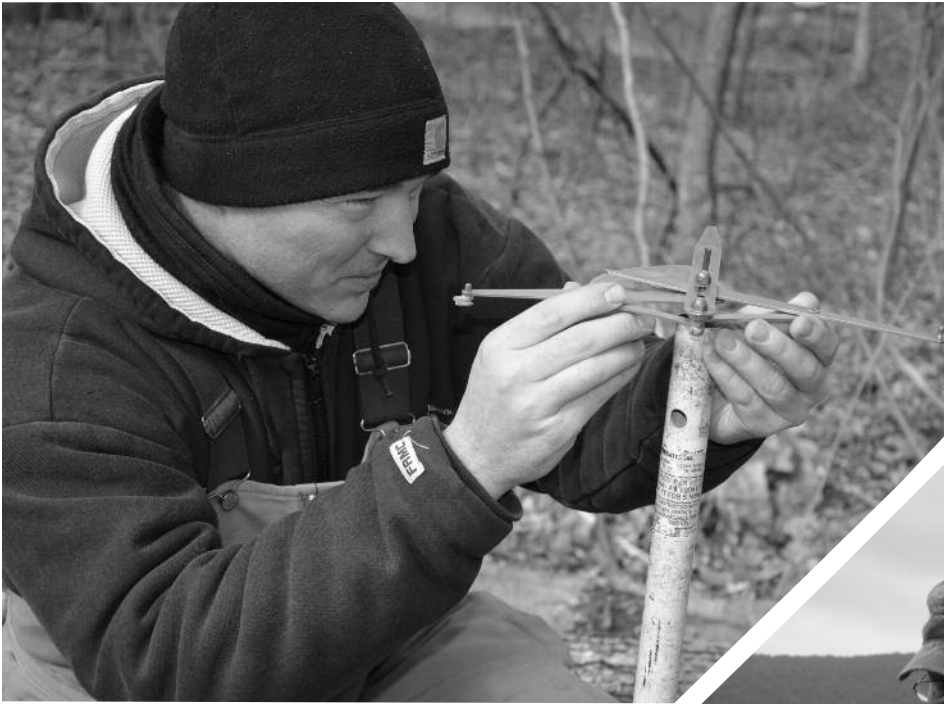
Above: Staking engineer Jason Hey uses a transit to select the route of a new line through a right-of-way. At right: Mike Lansberry uses GPS technology to plot a service drop to a turkey barn being built near Marklesburg, Huntingdon County in September. The GPS antennae is on top of his hat. (Photos by Doug Roles)
