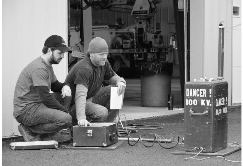
Josh Salyer (above, right), a certified non-destructive testing technician with American Test Center, and Cory Laib, a technician in training, monitor the testing of insulation in the boom of a bucket truck. Below: Technicians attach electrodes to each end of the boom. Photos by Doug Roles
