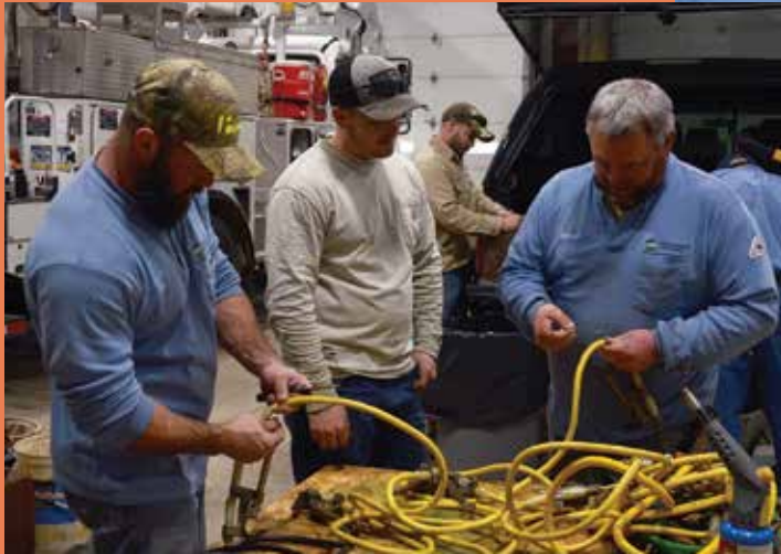
Our line crews tested their grounding equipment in February with the assistance of Pennsylvania Rural Electric Association safety instructor Randy Hoover. The safety event included classroom instruction on proper grounding procedures and inspection of all cables. Above: Hoover, left, and lineworkers Seth Glover and John Fogelsonger check resistance using a protective grounding set tester. At left: Eric Yingling, left, Glover and Rich Sunderland prepare cables for testing.
