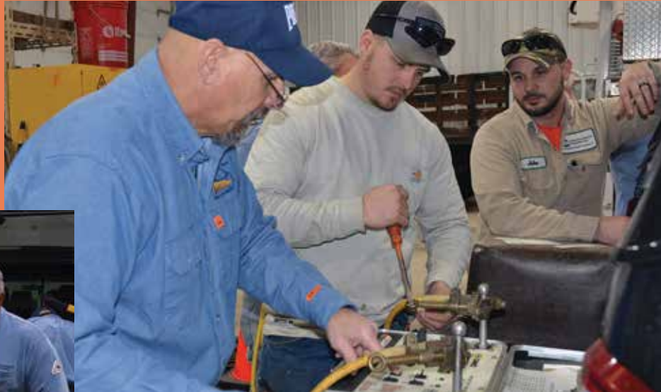
Our line crews tested their grounding equipment in February with the assistance of Pennsylvania Rural Electric Association safety instructor Randy Hoover. The safety event included classroom instruction on proper grounding procedures and inspection of all cables. Above: Hoover, left, and lineworkers Seth Glover and John Fogelsonger check resistance using a protective grounding set tester. At left: Eric Yingling, left, Glover and Rich Sunderland prepare cables for testing.
