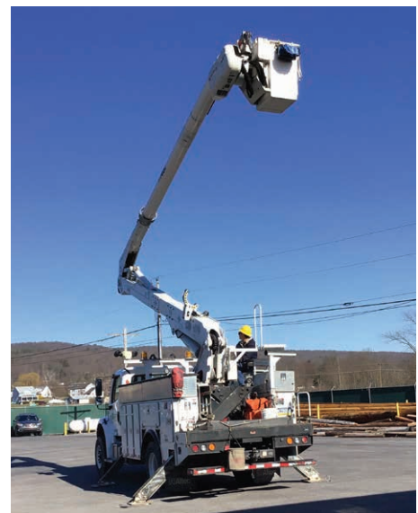
PREFLIGHT: A lineworker performs a preflight inspection on the aerial lift portion of a bucket truck prior to leaving the office.
